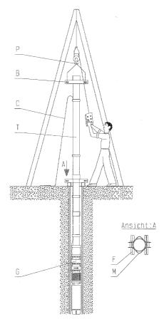
The suspension point (P) for the lifting gear and the support cable on the unit must be positioned so that the unit can be lowered centrically in the well or bore hole and that the unit will hang in exact vertical position.
