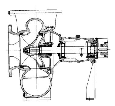
Casing pressure max. 10 / 16 bar (145 / 230 psig)
