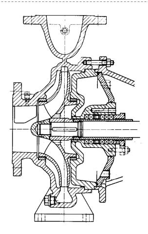
Stuffing box optional with cooling for temperatures up to 180 °C (350 °F)
