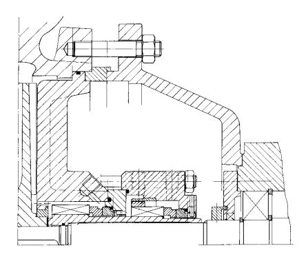
Double mech. seal in "tandem" arrangement acc. to EN 12756 (DIN 24960) with shaft sleeve, unbalanced optional balanced.
