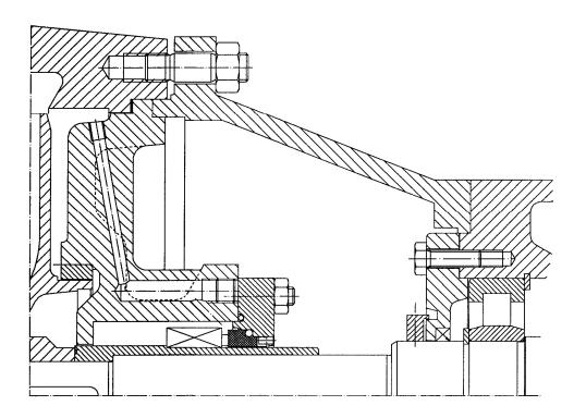
Inner single mech. seal acc. to EN 12756 (DIN 24960) with shaft sleeve unbalanced
