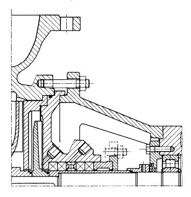
Hydrodynamic shaft sealing with expeller and stuffing box with clean water flush as stand by seal.
