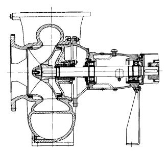
Horizontal single stage volute casing pumps with closed semi axial impellers
