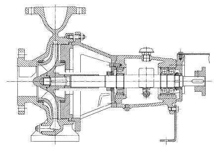
Shaft sealing: Stuffing box with internal or external sealing, flushing or cooling, hydrodynamic shaft sealing, mechanical seal acc. to EN 12756 (DIN 24960), inner single mechanical seal, double mechanical seal or Cartridge mechanical seal
