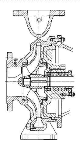
Stuffing box optional with internal or external sealing or flushing temperature up to 140 °C (280 °F)
