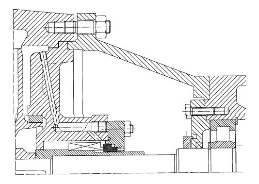
Inner single mech. seal acc. to EN 12756 (DIN 24960) with shaft sleeve, balanced design
