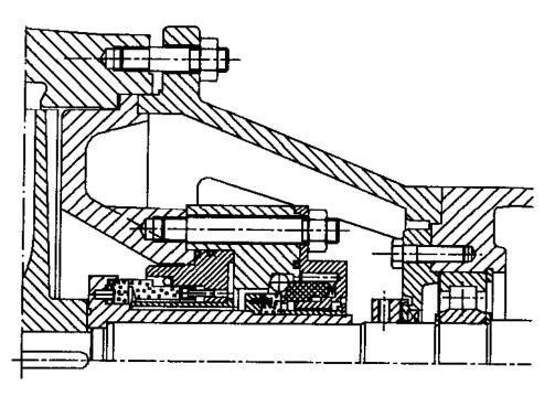
Cartridge mech. seal in single seal design. Optional in single seal design with quench. Optional as double mech. seal.
