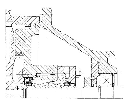
Double mech. seal in "back to back" arrangement acc. to EN 12756 (DIN 24960) with shaft sleeve, unbalanced
